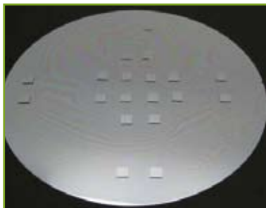
Figure 7: die to wafer structure after oxide interfilling.
