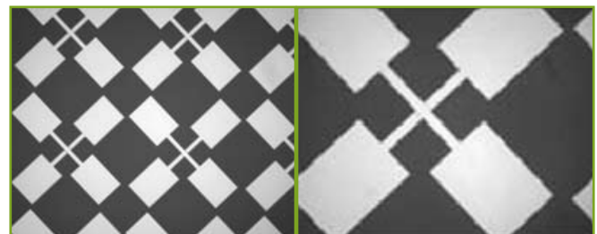
Figure 4 - Optical microscopy of the copper bonding Kelvin structure after silicon and silicon oxide etching. The pads are 95μm large and the bonded zone is 10x10 μm 2 .
